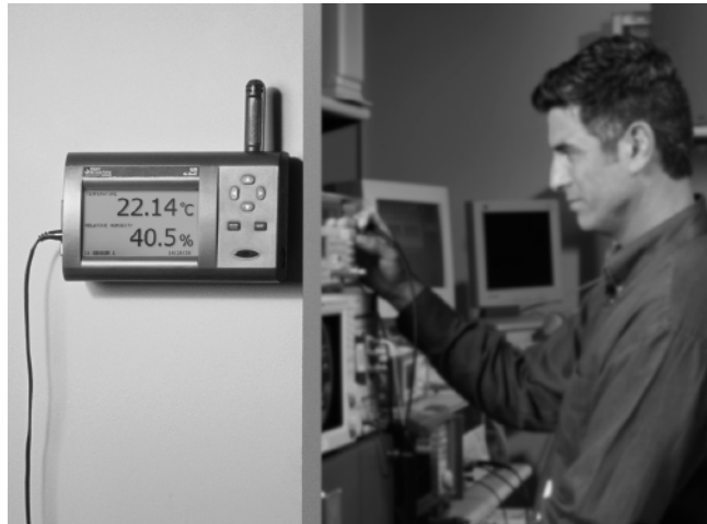
The DewK accurately records temperature to \pm 0.125 °C and humidity to \pm 1.5 % RH on two channels – with years worth of memory and multiple display options.
